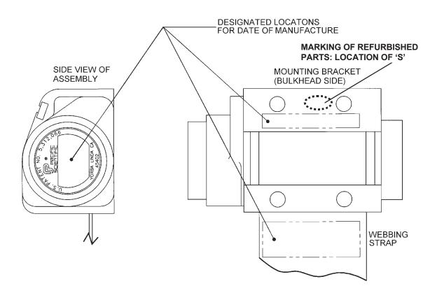
Figure 1. Location of Manufacturer's Date and Marking of Refurbished Parts
