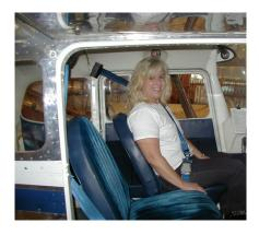
This structurally integrated Alpha Aviation Inc. 3-point Diagonal Shoulder Harness installation STC kit is FAA / PMA using OEM quality AmSafe® restraint assemblies meeting TSO-C114. Shipped as a complete kit, this STC includes everything for the installation of shoulder harness restraints in the Pilot and Co-Pilot positions
